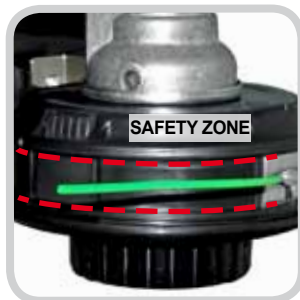
Locking hooks head outside the working area of the line.
